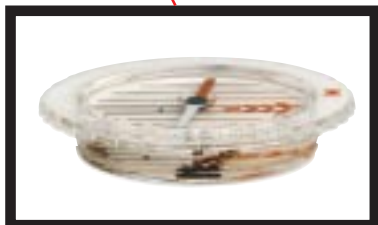
Ultrasonically welded, vacuum filled capsule with permanently clear anti-static liquid dampening. Needle swing stops in 4 seconds or less. Bubble free and water-proof. Proof tested from -40^{\circ} to +60^{\circ} .
